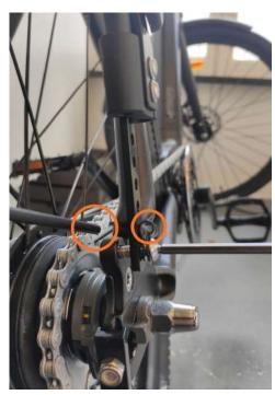
Now that the base of the carrier is fixed to the frame, it can be stabilized and brought into its final position. Start by removing the bolt that holds the middle of the rear fender. Then use this same bolt to attach the plate that will hold the stays / legs of the rack. Tighten it properly, it might bend inward slightly.
