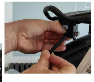
While taking a bird's eye view of the rear carrier, make sure it is perfectly aligned with the frame and tighten all bolts. This included the bolts under the plastic cover (see picture).
