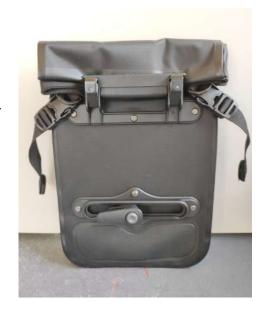
Simply hook the bag onto the side of the rear carrier as shown on the picture to the right. You should hear (and feel) a clicking once this is done successfully.
