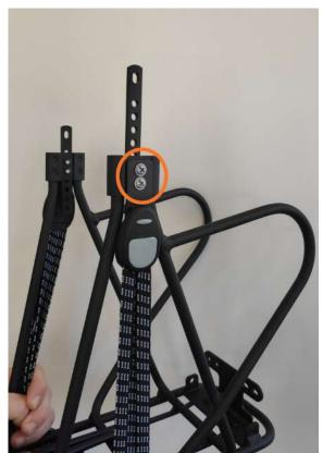
The rear rack will be fitted to the same bolt where your fender stays (that hold your rear mudguard in place) are currently connected to. Using a **4mm allen key**, remove these bolts on each side. Keep the fender stay bracket (circular clamps that hold the fender stay)
