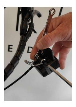
Then, install the lamp on the cap on your handlebar. Your choices in earlier steps will determine if the lamp will be located on top of the handlebar (such as in the picture to the right) or below.
