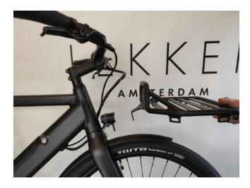
Please note: For the proper installation of the front rack, you need to remove the front light from its original placement and place it on the handlebar stem cap with light holder (see picture below). This cap is unfortunately only available from the 2nd week of August onwards. We will ship you the cap separately. Only once you receive this cap, can you install the rack and lamp correctly. We recommend waiting with the installation of your front rack until you receive this cap!
