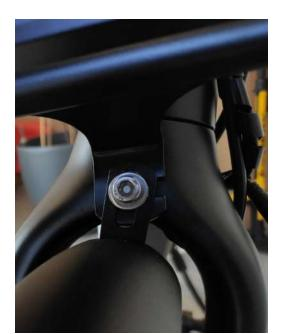
Now, attach the front carrier stays to the carrier using the provided bolt, nut and washers.
