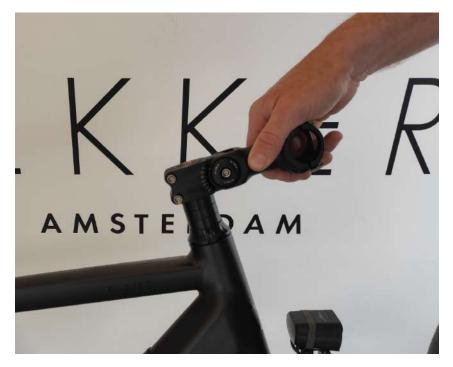
When tightening the new handlebar stem, make sure to tighten **the bolt on top of the stem** first. This bolt is necessary to connect the handlebar stem to the fork and the frame of the bike.
