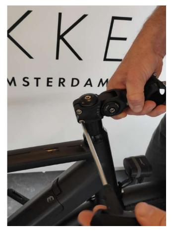
With the handlebar stem in a stable position, it is now time to re-attach the handlebar. For this, use the **4 mm allen key** to remove the four bolts on the front plate of the stem (see step 1). Check if the handlebar has the desired angle, then attach the handlebar and tighten those bolts to 5Nm.
