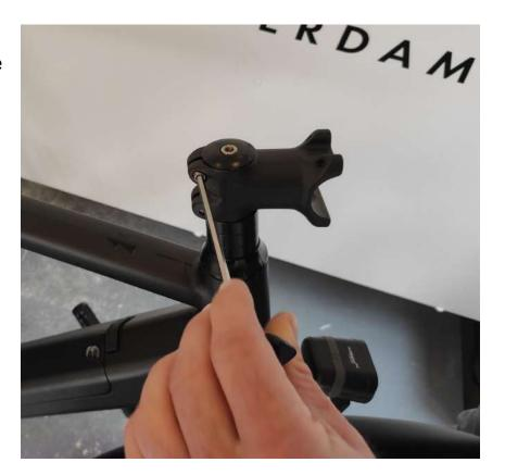
Now, with all bolts loosened, the handlebar stem can easily be removed from the frame of the bike.
