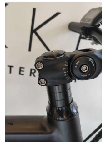
When the bolt is loosened, you can simply adjust the handlebar stem to the desired angle. Afterwards, strongly tighten the bolt to 12-13Nm.
