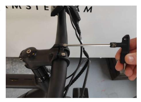
To remove the mounted handlebar stem, remove the bolt on the top using a **5mm allen key**.
