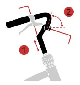
Tip: Should you wish to adjust the angles of you grips, brakes and shifter, you can do so with a simple turn of allen key 3 or 4. However, this should be correctly set already.
