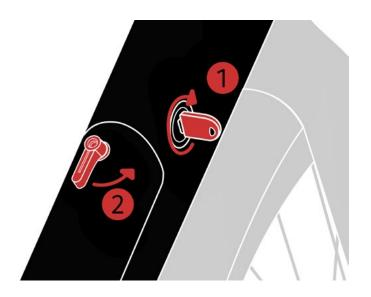
Step 2: After turning the key, the battery will partially pop out. Move the lever to fully release the battery.
