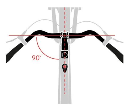
Tip: Should you wish to adjust the angles of your grips, brakes and shifter, you can do so with a simple turn of allen key 3 or 4. However, this should be correctly set already.
