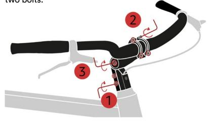
Step 2: To adjust the angle of the handlebar, use the same tool to loosen the faceplate at the front of the handlebar stem and reposition the handlebars. Then, tighten the handlebar to the stem with the four bolts.
