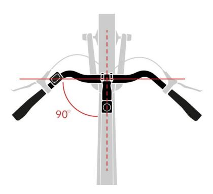
Tip: Should you wish to adjust the angles of your grips, brakes and shifter, you can do so with a simple turn of allen key 3 or 4. However, this should be correctly set already.
