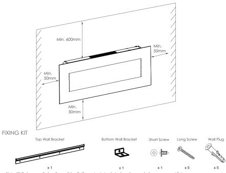
Note: Wall plugs supplied are for a solid wall. If screwing in to plaster board or wood, please use correct fixings.
