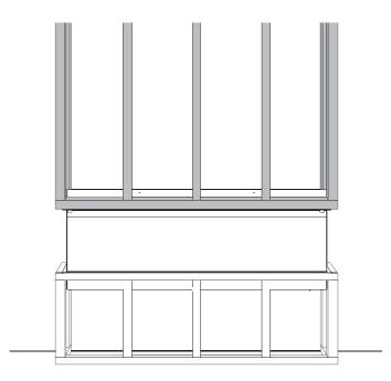
Board the wall/chimney breast with chosen material i.e. plaster board, MDF, etc.
