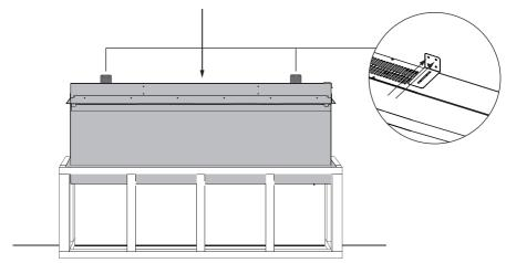
When fire is in place, construct the frame for the top half of chimney breast.
