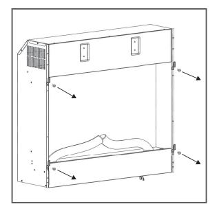
2. Tilt Firebox and insert into wall. Sit the Firebox on the ledge/stand central to the opening in the wall
