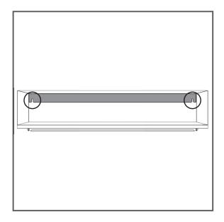
Then, push the trim onto the Firebox so it is flat against the wall.
