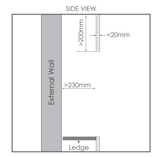
Behind the wall, a ledge must be positioned at the bottom of the opening for the firebox to sit on.
