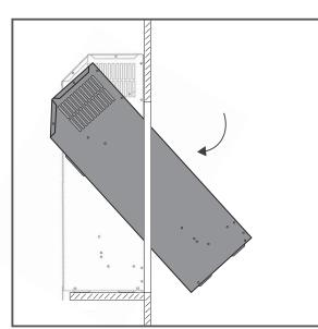
3. Once in the wall, locate the 2 x fixing brackets and fix to the firebox using 4 x screws removed from the metal tabs.
