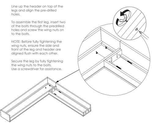
2. Repeat step 1 with the other leg, again ensuring the side and front of the leg and header are aligned flush with each other before fully tightening the wing nuts on to the bolts.
