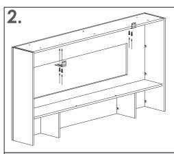
Using the 4 x small screws supplied, turn the brackets from the fire around and fix to the UNDERSIDE of the base top. Use the pilot holes to locate the brackets.
