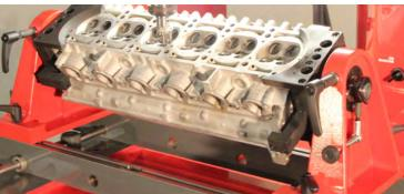
This feature (optional) allows a quick and easy mounting of the cylinder head while keeping a powerful clamping thanks to two jaws. It makes easier operations which require the access to different sides of the head.
