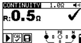
Figure 5.16: Example of continuous resistance measurement
