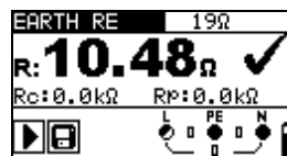
Figure 5.47: Example of earth resistance measurement result
