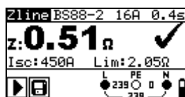
Figure 5.41: Examples of line impedance measurement result
