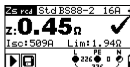
Figure 5.37: Examples of loop impedance measurement result
