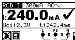
Figure 5.32: Trip-out current measurement result example
