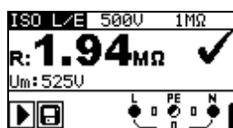
Figure 5.7: Example of insulation resistance measurement result
