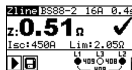
Figure 5.41: Examples of line impedance measurement result
