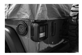
**Step 9** Attach strap around spare tire. Buckle and secure. (Same for 2 door versions)
