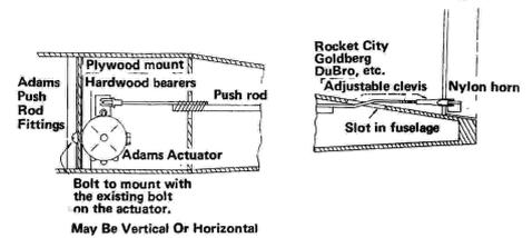
Bolt to mount with the existing bolt on the actuator.
