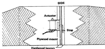
Motion of the actuator is carried to the rudder by means of a torque rod. At the rudder the torque is converted to right-left movement by a yoke fastened to the rudder. The rod should be light and rigid; construction can be of small dowl or square balsa stock with .045 piano wire on the ends. The piano wire is fastened to the dowl or balsa by wrapping with heavy thread and gluing. In smaller aircraft, the torque rod may simply be a piece of .045 music wire if the length is only around 6-10".
