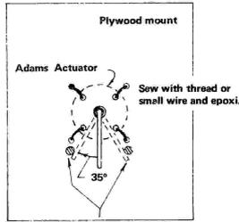
Stops to limit the throw of the actuator to 35° on either side. Make out of small dowel and glue in hole drilled into the plywood mount. A round toothpick works well.
