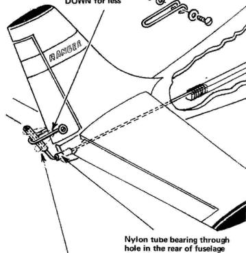
Bend end of torque rod after inserting in fuse. Heatshrink tubing over wire to prevent metal contact.
