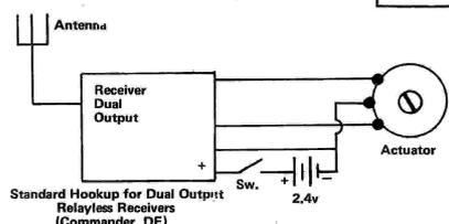
The use of nickel cadmium rechargeable batteries is most highly recommended. Any other types have proven impractical because of the amount of current drain the actuators employ. While they have been used successfully, in most instances they have given problems because they do not have the capacity of the nickel cadmiums, and they require replacement quite frequently and therefore in the long run prove much more expensive.
