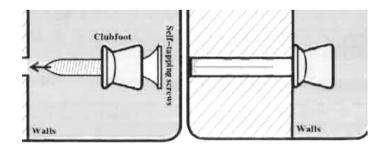
4. Fix 4 feet to the clubfeet, screw up the feet with a wrench until totally fixed.
