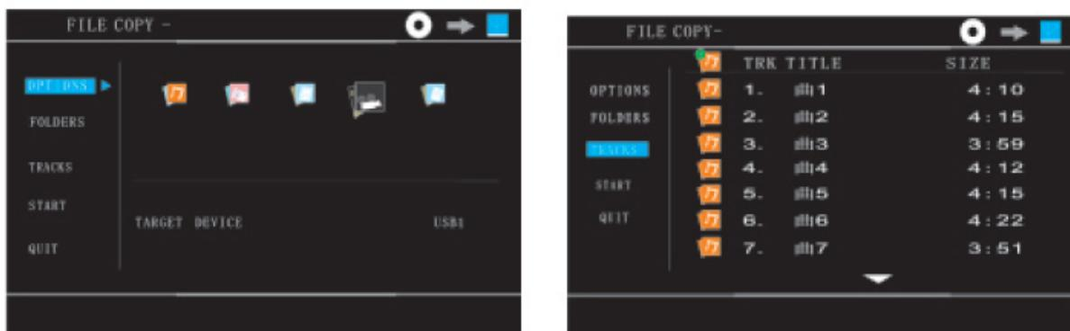
Press the enter button on the remote control to choose the desired music track, press the arrow buttons on the remote control to move the cursor to the START option and then press the enter button to start copying.
