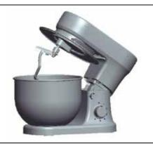
4. Turn the attachment, so the pins on the spindle are aligned with the depressions on the attachments top edge. Press the attachment against the swivel arm and turn it anti-clockwise at the same time until the pins engage and the attachment locks into position securely. The attachment must not be loose, nor should you be able to pull it free.
