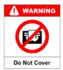
WARNING: FIRE RISK EXISTS WHEN THE HEATER IS COVERED BY OR POSITIONED CLOSE TO CURTAINS OR OTHER COMBUSTIBLE MATERIALS.
