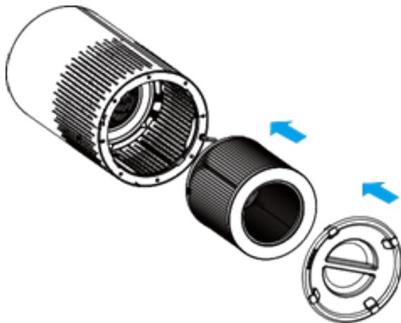
5. Turn the base cover clockwise from OPEN position to LOCK position, you will hear a "click" sound, the base cover is fastened.
