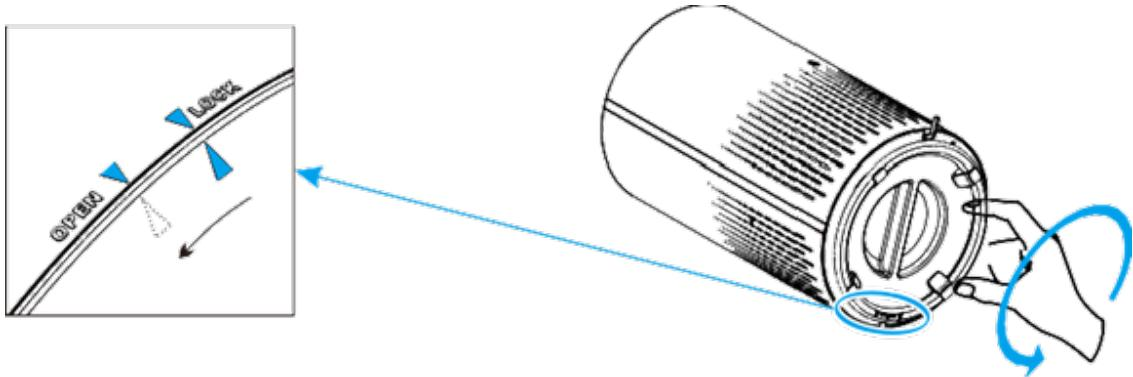
2. Remove the base cover and take out the filter.
