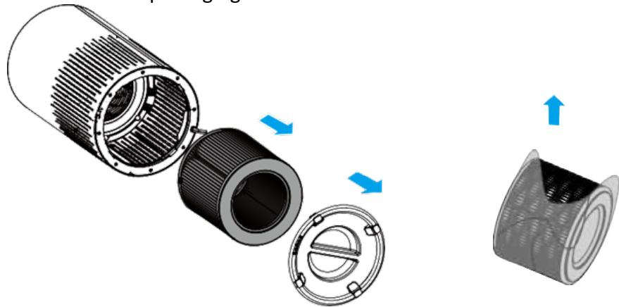
4. Put the filter back into the air purifier.
