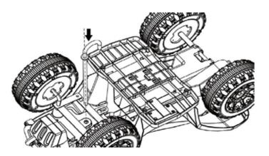
4. Turn the ride on bottom up. Insert the steering shaft.
