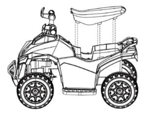
Connect the large connector underneath the seat to the corresponding connector from the gear box motor.
