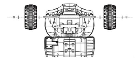
2. Add the front wheels, gaskets and nuts as pre the diagram above to the front of the ride on.
