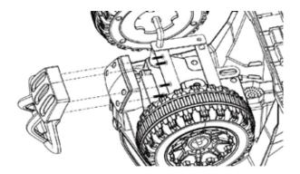
3. Add the front bumper. Use 4 x "4 X 10" screws and a screwdriver (not included).
