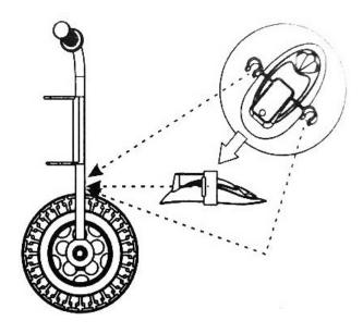
Add the front wheel cover by clipping it onto the fork above the front wheel.
