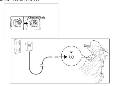
Insert the plug of the charger into the charging socket which is on the main body of the bike below the siren and music buttons.
