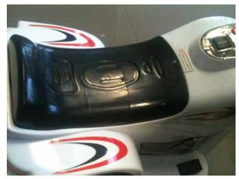
To access, remove the screw using a screwdriver (not included) holding the heat down and then take the seat off the body.
