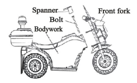
Join the main body of the motor tricycle to the front end with the front wheel using the bolt and washer and nut included.
