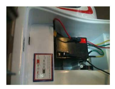
Plug the red connector onto the red terminal of the battery. Plug the black connector onto the black terminal of the battery.
