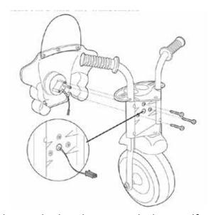
Fix the windshield onto the head cover with three self-tapping screws.
