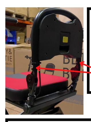
Locate the back of the seat on the mobility scooter and look for these screws highlighted. They are the ones directly under the backrest.
