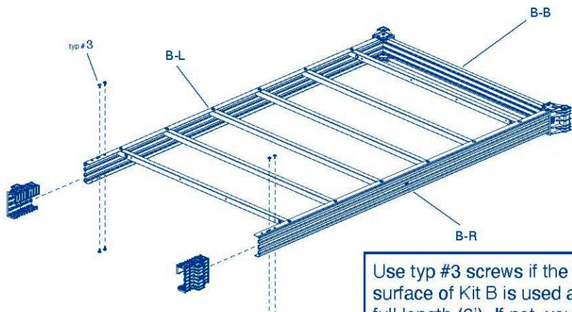
Use typ #3 screws if the table surface of Kit B is used at its full length (6'). If not, you need to use the typ #7 screws instead of the typ #3 screws.
