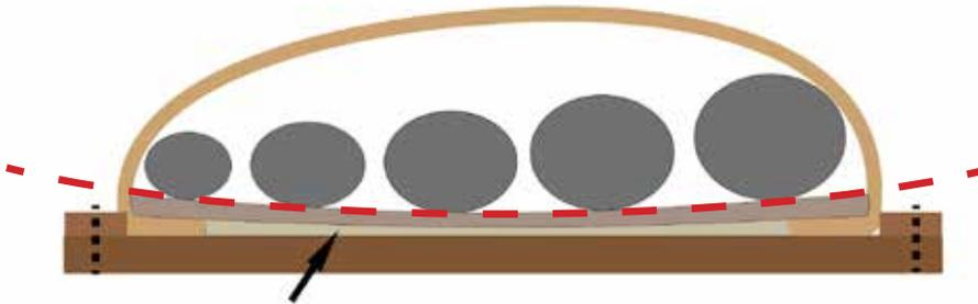
Direct Injection, Storzbel or Cemented Construction
