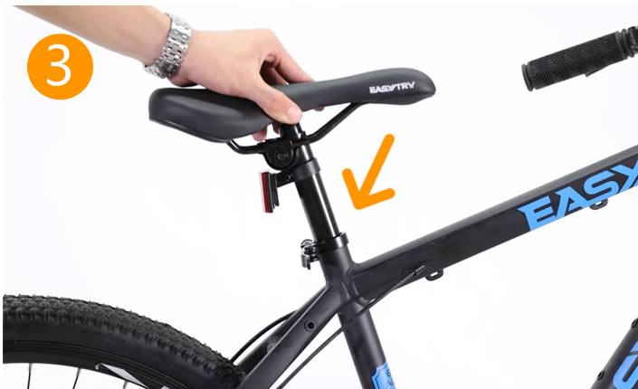
Put the saddle into the riser and tighten
