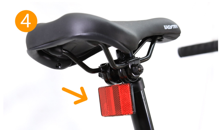
Adjust the position of the reflective warning board
