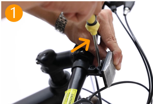
Adjust the reflective warning board to a suitable position
