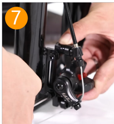
Tighten the second screw
