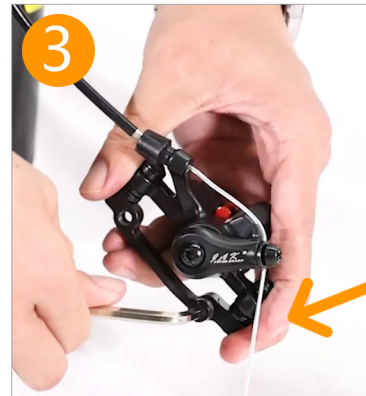
Unscrew the 2 screws that fixed on the front caliper
