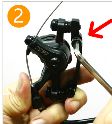
Unscrew the 2 screws that fixed on the front caliper
