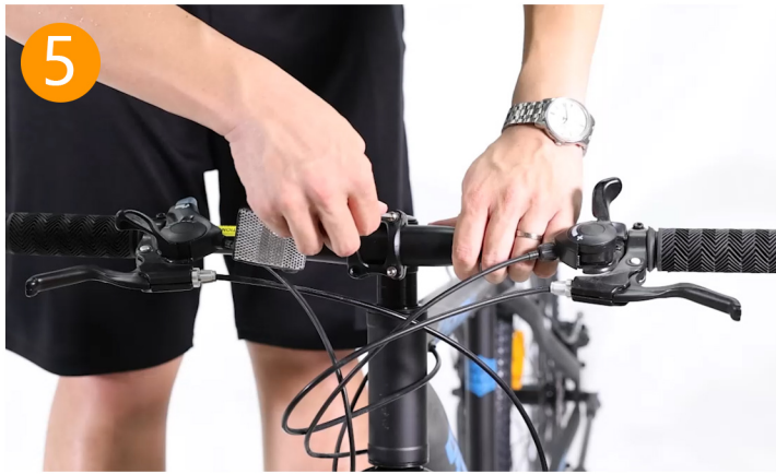
Then tighten the 4 screws
