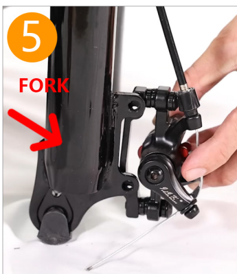
Align the hole of the brake caliper with the hole of the front fork
