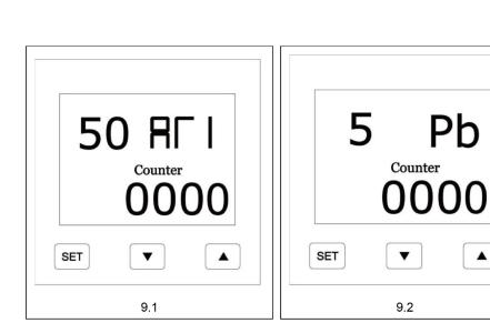
if temperature on heater is higher than circuit board shows,pls raise the Pb
