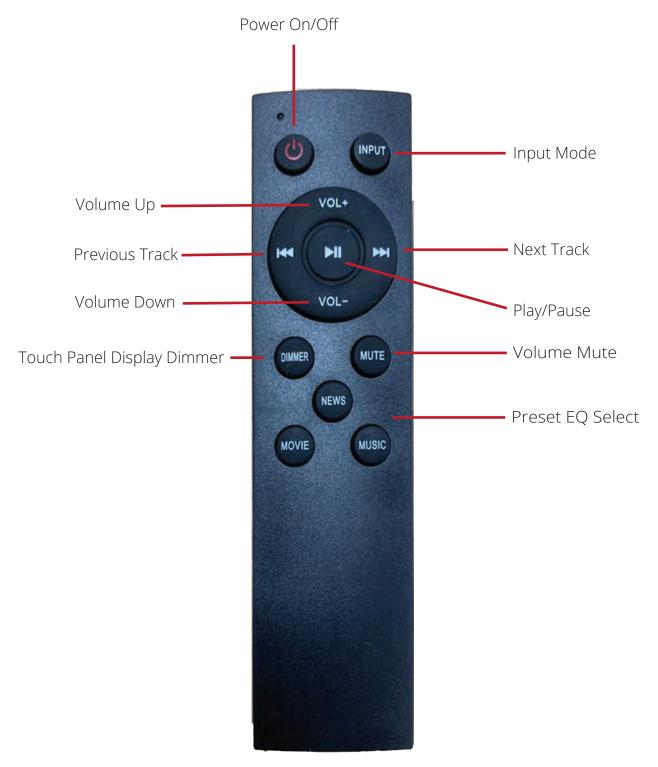
The uStream One system can be controlled from the touch panel on the top of each speaker or via the included remote control handset.
