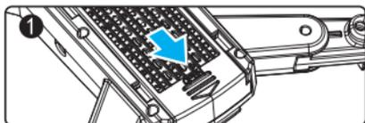
6.1 Slide the battery cover open according to the arrow direction
