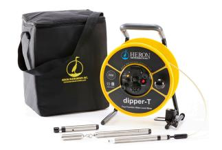
The Well Casing Indicator Probe is used to measure the depth of metal casing in wells and boreholes from two inches in diameter and upward. The Well Casing Indicator Probe works using magnetism. While the probe sits within the magnetic field of the steel casing, an auditory and visual signal is active. When the probe leaves the magnetic field the signal stops. Note the condition of the well for accurate readings.
