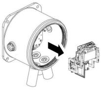
When the captive screws are completely loose, grip the sides of the frame of the Detection Module, as shown, to remove it from the Housing Module.
