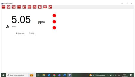
This tab displays in real time what is displayed on the Titan 2 screen. A radio button allows the user to switch between the current cycle reading and the calculated STEL.
