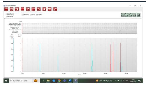
Hold down the left mouse button to grab and drag the graph around the screen. Use the mouse wheel to zoom in and out.
