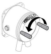
Turn counter-clockwise to unscrew the front cover.
