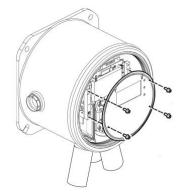
Use the four screws to attach the face plate. Tighten them firmly hand-tight.
