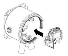
Hold the ribbon cable out of your way while you insert the Detection Module.
