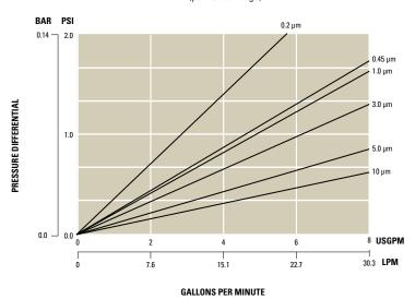
For liquids other than water, multiply the pressure drop by the fluid viscosity in centipoise.
