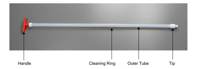
Diameter of Outer Tube: 25mm
