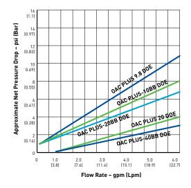
Change-out frequency will depend on the oil burden in the application. Because no appreciable increase in pressure drop is observed during service life, the filter must be changed when its adsorption capacity is exhausted.
