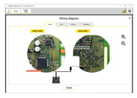
Once ready with the connections you can proceed to reading the unit by pressing the "Read MCU" button. Once the unit is read, the software will display the available information and you will see a screen like the one below (note that in this case we are using Renault HFM; Other units will display different information)
