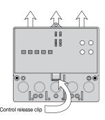
Press the control release clip on the base inside the wiring chamber and slide the control upwards.
