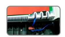
Make sure to put the wires through the grooves.
