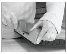
Insert screwdriver and push tab inward, cover should release from base.
