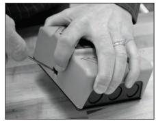
Turn box and repeat inserting screwdriver and pushing tab inward on opposite side, cover should release from base.
