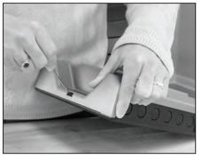
Hold either the left or the right end of the box up and at an angle. Use body for stabilizing relay box.
