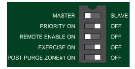
TSTAT 1, ZONE 1 will operate as priority and all other zones are temporarily switched off (with 1 hour time-out). When priority is OFF, any zones that were active when ZONE 1 was switched on will remain on.
