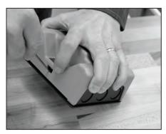
Hold either the left or the right end of the box up and at an angle. Use body for stabilizing relay box. Insert screwdriver and push tab inward.
