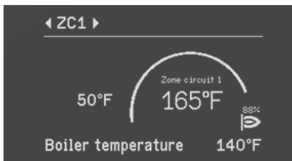
Zone control interface
