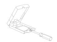
If necessary, mark and drill the appropriate fastening holes using the installation template. If needed, use the wall anchors included.
