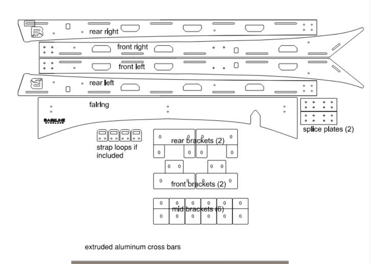
Please note that Aluminum may bow when cut from panels or when heated during the powder coating process. This won't affect the performance or look of your rack, and it will straighten out when it is assembled with the cross rails. If bowing is present it is recommended to arrange the side sections to oppose each other like ( ) or ) (
