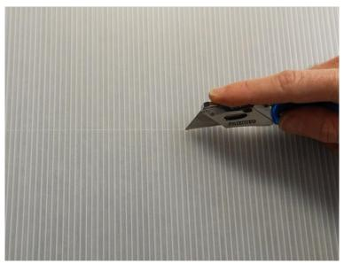
On the first pass, use light pressure to score the panel and set the path the knife will follow for the second pass.
