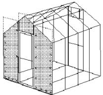
NOTE: When trimming off portions of Solexx paneling during the end wall paneling installation, you should leave an extra 1/8" (3mm) of the paneling above the framing that you are using as a cutting guide. This allows the end wall paneling to "snug" up against the side walls and roof paneling. Once the paneling is attached and trimmed seal any of the open ends of the paneling with 100% Silicone caulking.
