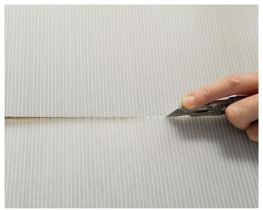
The second pass should be done with more pressure to cut through the panel, while making sure the knife is following the score line of the first pass.
