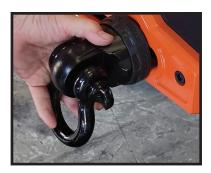
Lastly, install shackle to aluminum shackle body. Winch in to secure shackle mount in to place firmly against fairlead.
