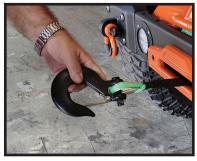
To install, remove old hook. On most hooks, you will need to remove cotter and pin to remove from cable or rope. Some hooks you will have to cut.
