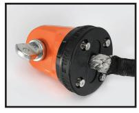
Slide backing plate over aluminum shackle mount. Line up the 4 allen holes. Securely tighten the 4 allen screws.
