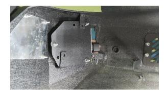
**Step 4:** Bolt the plate to the bumper brackets with the 2 bolts, washers, and nuts using a 4mm hex key and 10mm socket. (Adjust the bracket around to make sure (1. The sensor in centered in the hole, 2. The wire has enough clearance from the front of the bumper and the bumper bracket.))
