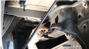
Remove both of the shown brackets with a 12mm socket.
