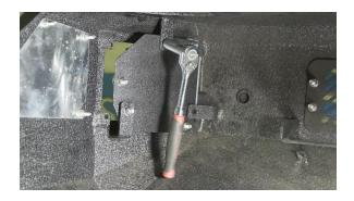
**Step 5:** Install the plastic plate on the outside. Bolt the plastic plate in with the 4 bolts, washers, and nuts using a 3mm hex key and 8mm socket.
