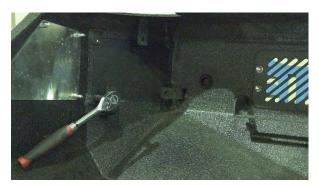
**Step 2:** Find the plate for the correct side (shown is the plate for the passenger side). Install the sensor into the plate as shown with the 3 supplied M5 bolts, washers, and nuts. Using a 4mm hex key and 10mm socket snug up all 3 nuts. (The holes in the plate allow for movement to adjust the sensor in the right position).
