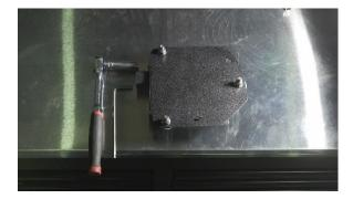
**Step 3:** Slide the plate and sensor behind the bumper brackets. At this point the sensor should be connected to the wiring harness.
