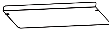
Indoor baffle (required for air exhaust outside, not required when exhausting inside)
