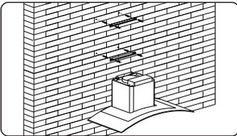
Mark down the position and drill 2 holes for each chimney bracket and tighten the bracket with screws.
