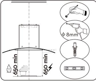
Prepare pencil, electric drill, plastic wall anchors and level before installation. Recommended installation height: 700mm. Required minimum installation height: 650mm.
