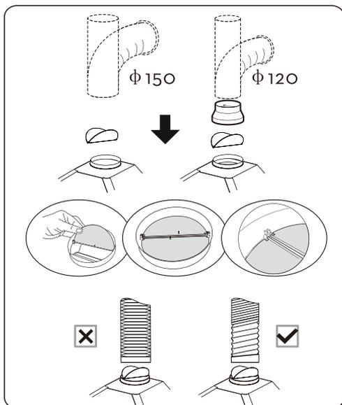
**Installation method for 150mm diameter pipe:** insert the one-way-valve as the pic and fix the pipe.
