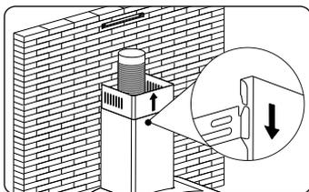
Put the upper chimney into lower chimney . Then pulling out the upper chimney upwards. Adjust to reach the height required.
