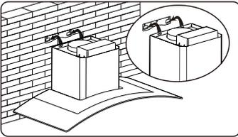
Lift the cooker hood and hang onto the wall hook.
