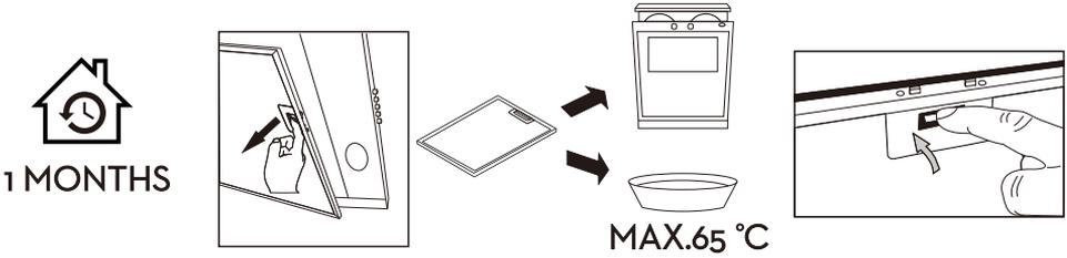
**Aluminium filters:** To avoid fires, clean thoroughly once a month or whenever the display pilot lights up (if fitted). To do so, remove the filters and soak in hot water and detergent for an hour. If using a dishwasher, position the filters vertically to improve the cleaning process.
