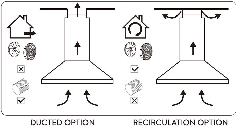
a.If you have an outlet to the outside, your cooker hood can be connected as above picture by means of an pipe (with an interior diameter of 150mm). If you don't have an outlet to the outside, you can go with recirculation mode by using carbon filter.
