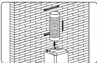
Fix the one-way-valve to the air outlet of the cooker hood, and then attach the pipe onto the air outlet as picture.
