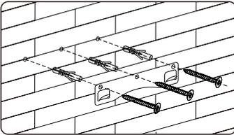
Drill  $3 \times 8\text{mm}$  holes to accommodate the bracket. Screw and tighten the hook onto the wall with the screws & plastic wall anchors provided.
