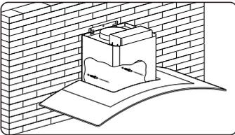
Need to drill  $2 \times 8\text{mm}$  extra holes & fixing screws & plastic wall anchors before installation.
