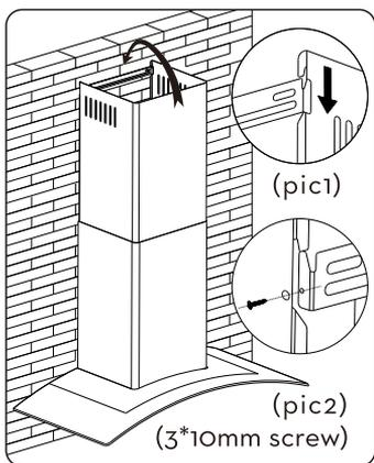
There are 2 methods for installing the chimney cover. Please check the attached pic for reference.
