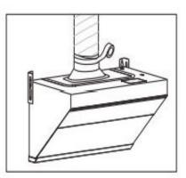
9. The range hood must be kept horizontal. The install the oil collector. Then plug into the power supply to test the range hood.
