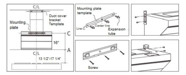
7. Lift the range hood horizontally and hang on the mounting plate on the wall. After the whole range hood is positioned, use 4X40mm wood screws to fix the steel angle brackets on the left and right sides to the wall. Lift the range hood horizontally and hang on the mounting plate on the wall. After the whole range hood is positioned, use 4X40mm wood screws to fix the steel angle brackets on the left and right sides to the wall.
