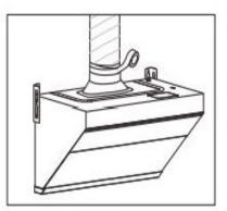
10.The range hood must be kept horizontal. The install the oil collector. Then plug into the power supply to test the range hood.
