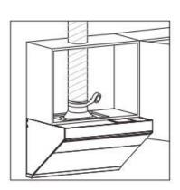
7. The range hood must be kept horizontal. The install the oil collector. Then plug into the power supply to test the range hood.
