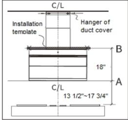
5. Take out the angle bracket template. The vertical center line in the template will align with the range hood center line, and the horizontal center line will align with the line B. Stick it flat on the wall, then drill holes in the drilling positions. and insert plastic expansion tubes in the holes, install 4x40mm screws.
