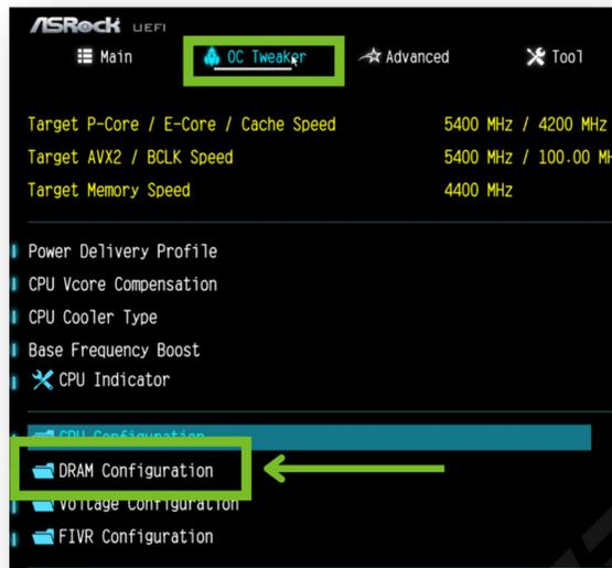
4. For the “Load XMP Setting” note whether XMP Profile is enabled.
