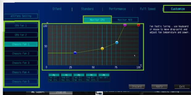
Ensure that you re-apply custom fan curves for every fan because some systems will have the Liquid Cooler Pump hooked up to a Chassis Fan Header.
