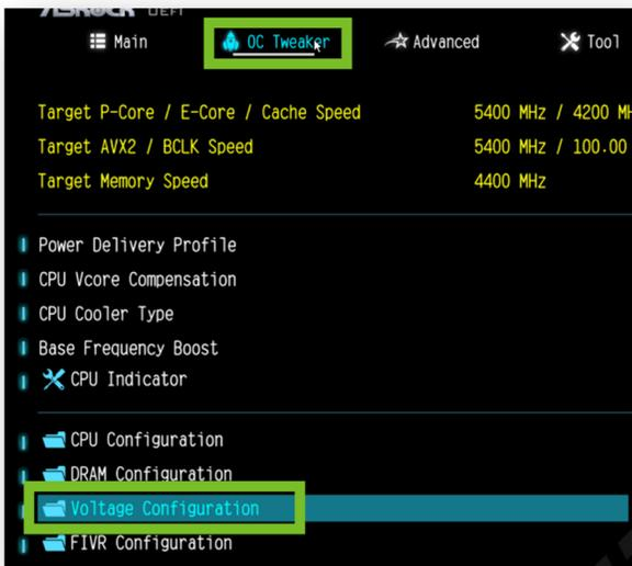
6. Within the voltage configuration, change the CPU Core/Cache Load-Line Calibration Settings to Level 3.
