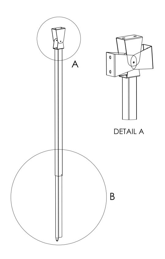
**NOTE:** Maintain 6.00" (minimum) of Channel length inside the Down Tube.
