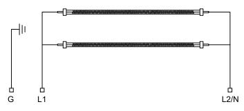
Enclosed 4' Whip is Supplied with Three High-Temp wires [1 Black, 1 Red & 1 Green (Ground) with Ring Terminal] installed in flexible metal conduit. Hi-Temp Ceramic wire nuts are provided.
